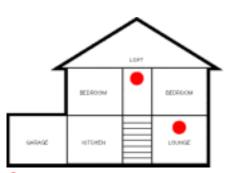
Minimum recommended locations for installing smoke alarms
